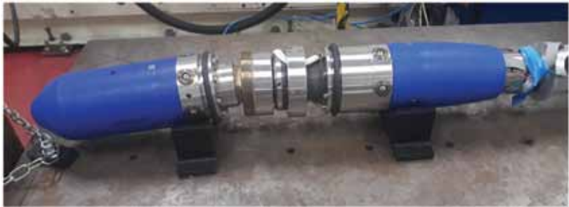
FIGURE 7 Photograph of the in-bore laser welding tool.
